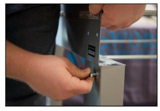
7. With the holes of the base and the leg aligned, insert a washer and a hex bolt into the outer hole.
