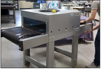
2. On the infeed side, take the other end of the belt and thread it under the infeed roller and under the lower cross brace, through the lower slot on the roller/rail assembly. Guide the belt through the oven chamber so it continues through the lower slot and over the lower cross brace.
