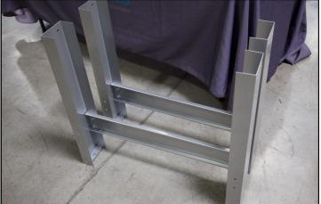
5. Repeat steps 1-4 to build the other two legs and cross brace. These are the legs that the body of the dryer will attached to.
