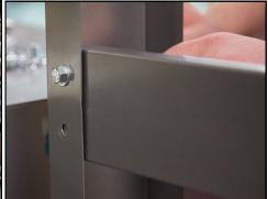
2. Insert a washer and a hex bolt  $(3/8-16" \times 3/4")$  into the top holes. Hand tighten a lock nut onto the other side of the bolt.
