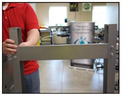
3. Insert washers and hex bolts into the two holes for both legs. Hand tighten lock nuts onto the backside of every bolt.
