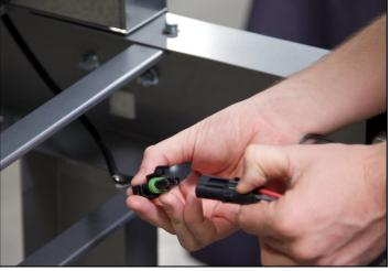
4. Connect the plug located inside of the machine to the plug attached to the motor located on the arm.
